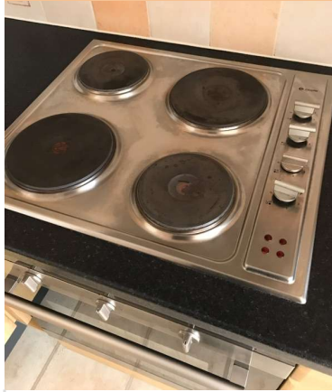
Rust signs on hob
